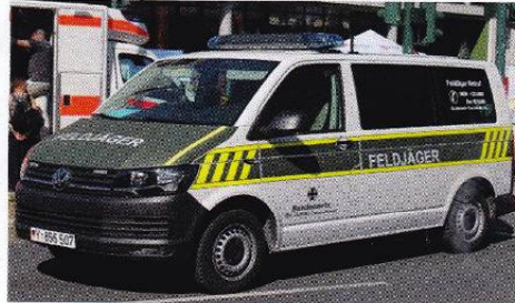
Volkswagen T6 Feldjäger, 110 kW, 150 PS, max. 182 km/h, Rundumkennleuchte Blau
