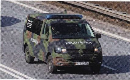
Volkswagen T6 Wipper, 110 kW, 150 PS, max. 150 km/h, Rundumkennleuchte Blau
